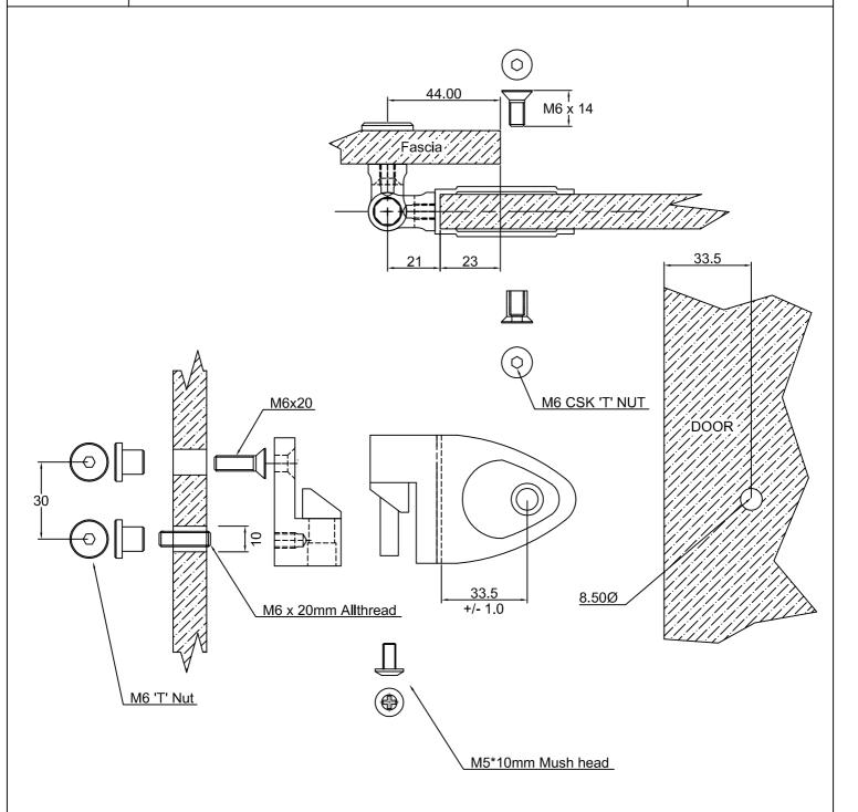
The hinges are secured to the panels by 'T' Nuts, Allthreads and Machine Screws. The drilling details are laid out in the detail of this sheet and the following page.
